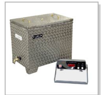
FZ-31A Steam Tank for Cement
