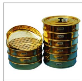
Laboratory Analysis Sieves for Soil and Rock Testing (made of brass)
